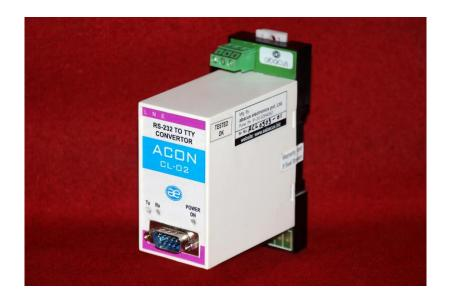
**INTRODUCTION:** The model ACON CL-02 is RS 232 to current loop (TTY) converter. This is 20mA current loop suitable for distances upto 1.2 Km. over two twisted pair. The optical isolation protects one segment of your network from problems that arises on the other.
